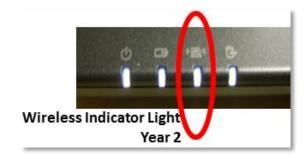
To turn the 'Wireless Network Switch' back on, press the 'Wireless Network Switch' button on the top row of the keyboard on *year 1 netbooks* or slide the switch on the left front side on the *year 2 netbooks*. Check to see if you can now connect to wireless by opening Internet Explorer or Firefox.
